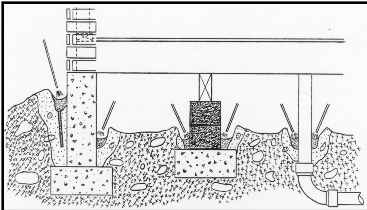
**Figure 2.** Rodding and trenching techniques are used around stem walls, footings, pier blocks and utilities to create an impermeable continuous barrier to guard against termite attack. A proper application will prevent the washing out of soil from under the support structures and prevents their settling into over softened soil.
